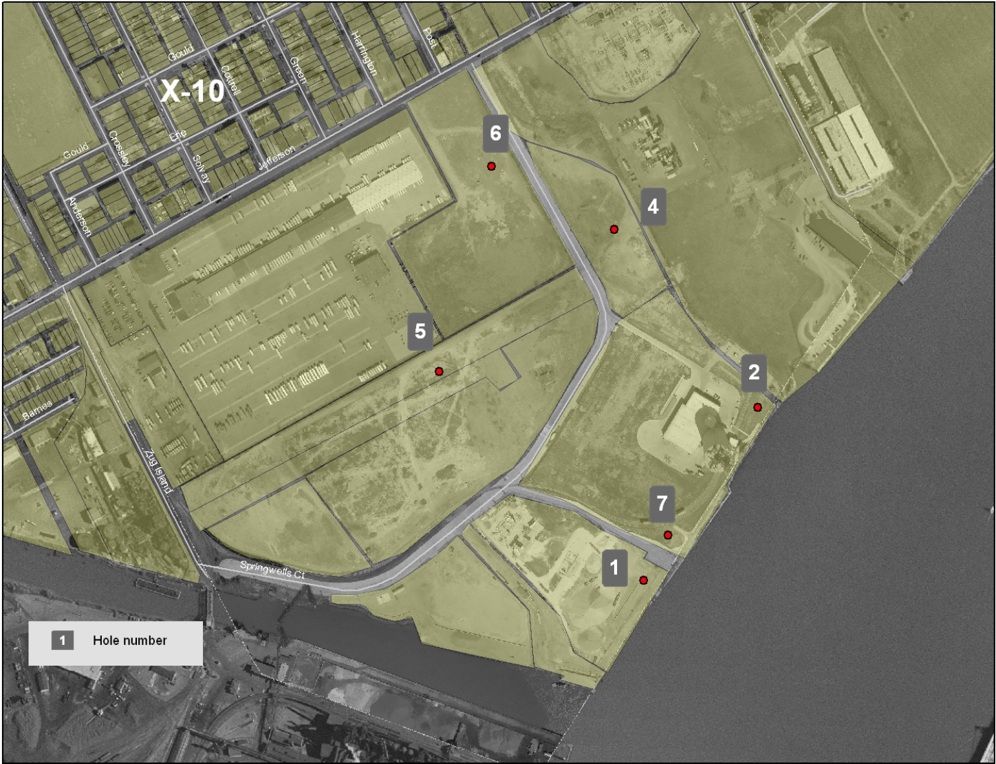
Figure 4-1 Detroit River International Crossing Study Final Test Boring Location Plan – Site X-10
