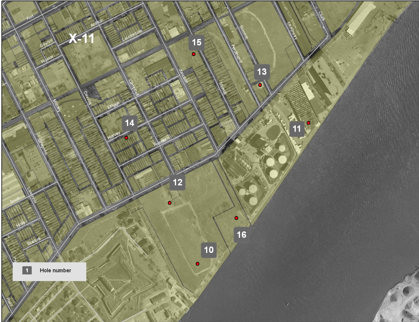
Figure 4-2 Detroit River International Crossing Study Final Test Boring Location Plan – Site X-11
